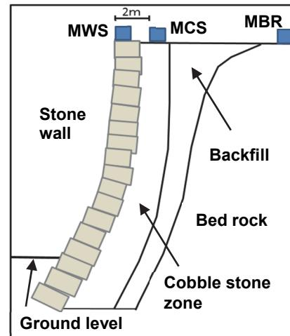
Fig. 3 Schematic of a cross section of a typical stone wall at the Marugame castle
