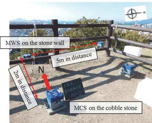
Fig. 4 Measuring by microtremors
