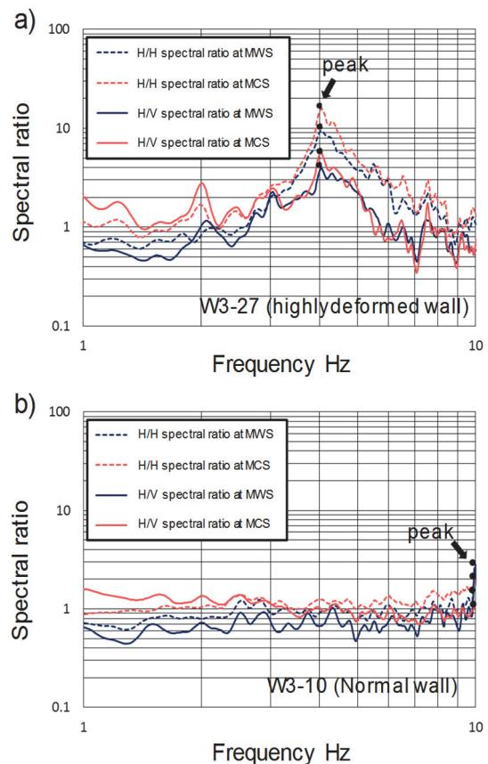
Fig. 6 Typical H/V and H/H spectral ratios obtained at W3-27 a) and W3-10 b)
