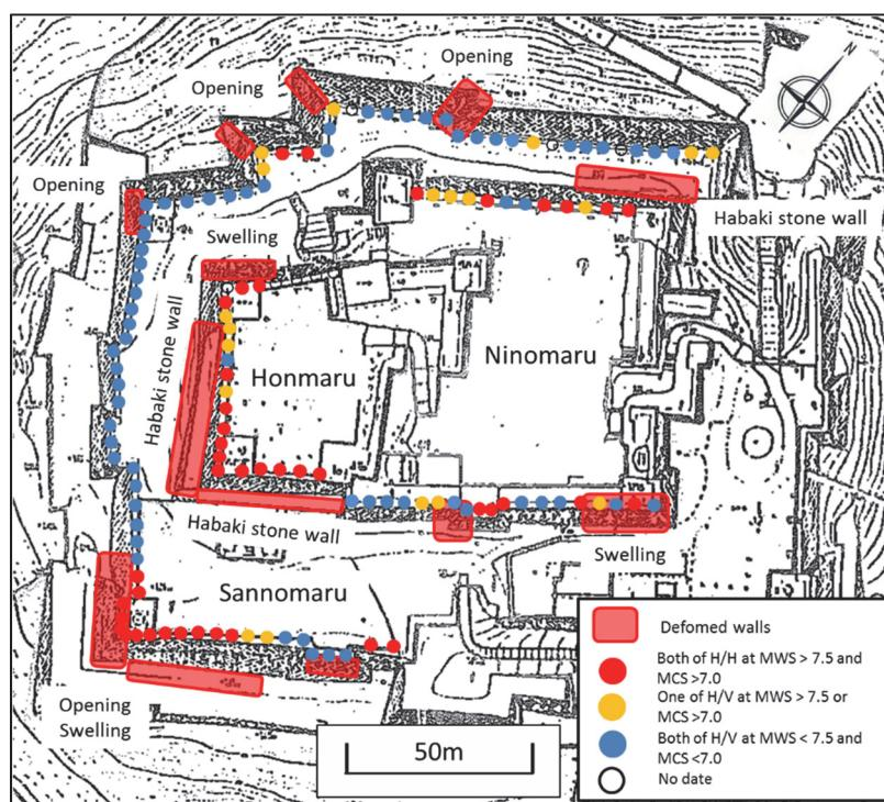
Fig. 11 Location of deformed wall and the distribution of the thresholded value of H/H ratio
