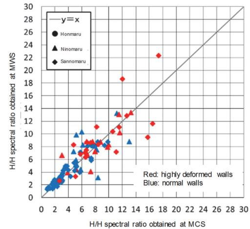
Fig. 9 H/H spectral ratio obtained at MWS and MCS
