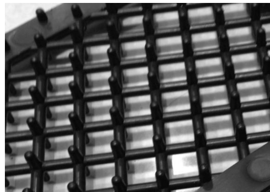
Fig.2 Disk of the rotating biological contactor
