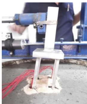
Fig.9 Gap occurred under cyclic loading
