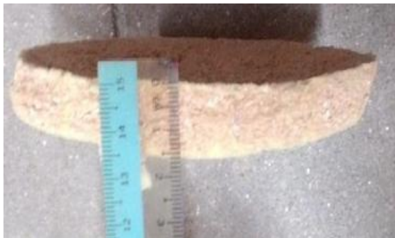
Fig 15: Polyurethane layer after test becomes thinner
