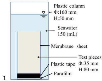
Fig. 2 seawater exposure test setup
