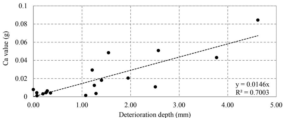
Fig.6 Relationship between Ca value and deterioration depth
