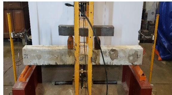
Fig. 4 Four-point bending test on a typical beam specimen
