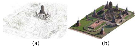
Fig. 11 The 3D point cloud, (a) Sparse point cloud, (b) Dense point cloud
