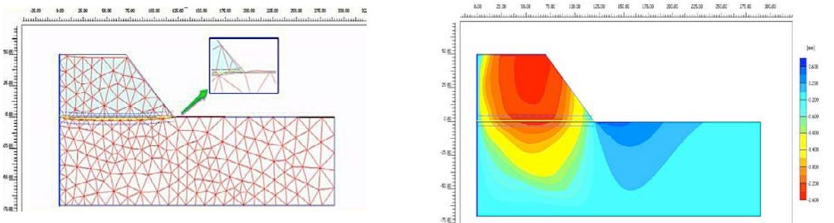
Fig. 6 Deformed mesh (b) vertical displacements (Case II)
