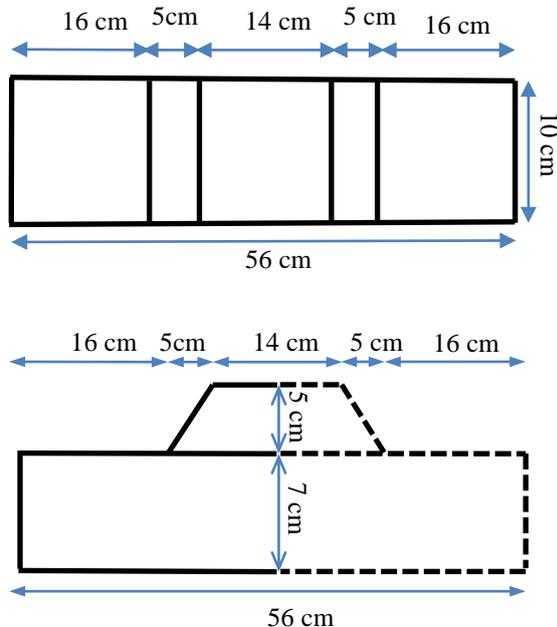
Fig. 1 Plan view and cross-section of embankment model
