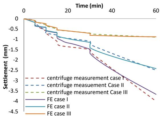
Fig. 9 Vertical displacement of different cases resulted in centrifuge test and FE analysis
