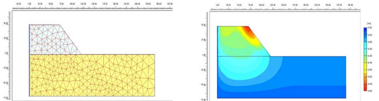
Fig. 7 Deformed mesh (b) vertical displacements (Case III)
