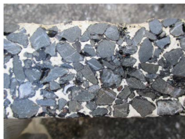
Fig.7 Injecting condition of the cement-based grouting material in JGZ-3 specimen
