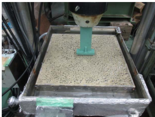
Fig.4 Specimen fixed in a water tank
