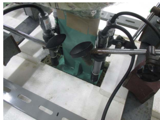
Fig.5 LVDTs attached onto the corners of the loading plate
