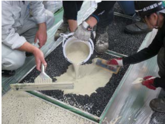
Fig.3 Cement-based grouting material poured into voids of the porous asphalt specimen
