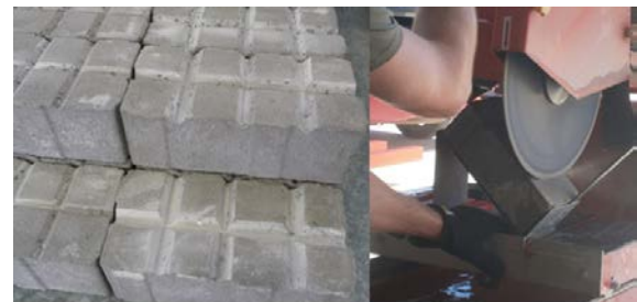
Fig. 7 – Sediment Slots Being Cut into Underside of PICP blocks [21]
