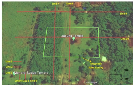
Fig. 4 Geoelectric, dipole-dipole configuration Line and Magnetic Measurement in Jabung Temple area
