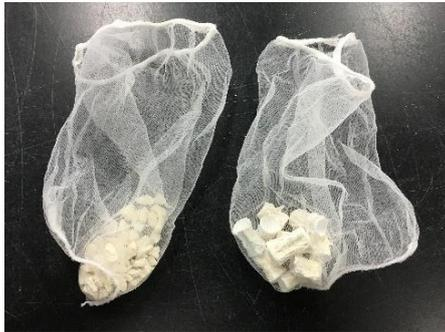
Fig. 6 Filter bag containing zeolite(left) or HAp (right)
