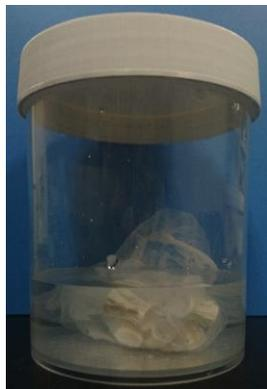
Fig. 7 Immersion test experiments to compare the performance of the HAp due to its ability to highly adsorb cesium [11].
