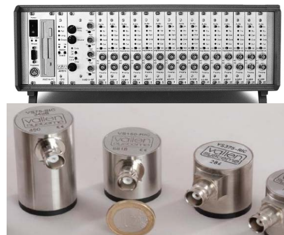
Fig. 10 AE Sensors and Multichannel processor of acoustic emission technology (Vallen).
