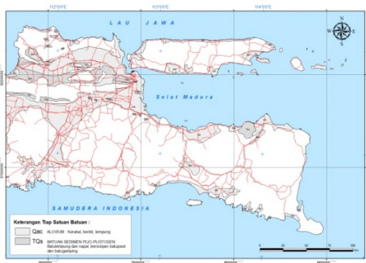
Fig.1 Map of the spread of soft soil and expansive soil in the northern part of East Java, Indonesia and transportation infrastructure (Rachmansyah, 2014).
