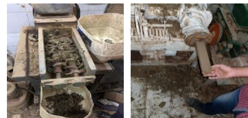
(a) Prototypes pressing machine (b) Brick production process
