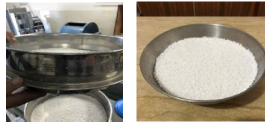
(a) Preparing the polyurethane foam sieve No. 2.76 (b) Final shape of the polyurethane foam
