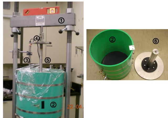
**Fig. 2.** Test setup for model pile loading test: ① Adjustable height loading frame ② Test tank ③ LVDT ④ Load cell ⑤ Model pile, ⑥ Compaction base plate.
