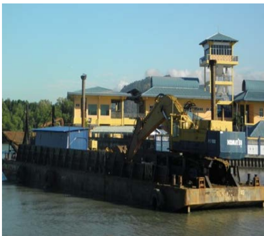
Fig. 1 Excavation dredger on the barge in Kuala Perlis, Malaysia
