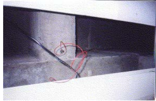
Fig.4 The situation of the sensors arrangement at the floor/beam structure
