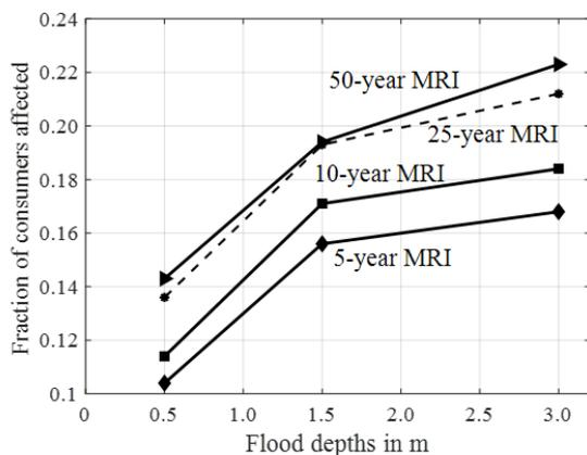
Fig. 5. Vulnerability curves for power loss
