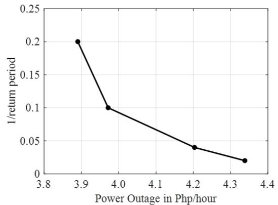
Fig. 6 Risk curve for power loss due to flooding
