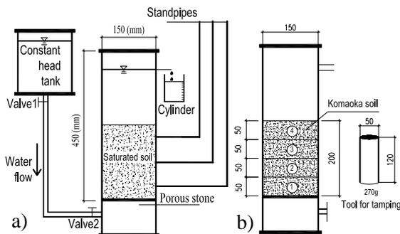
Fig.8 Schematic diagram of seepage flow test: (a) test apparatus ( $\phi 150\text{mm}$ ), (b) preparation of test specimen
