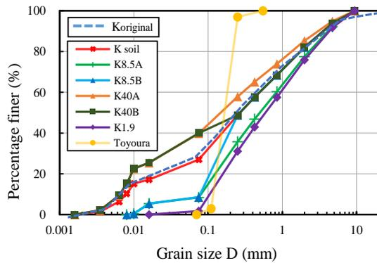
Fig. 2 Grain size distributions of test materials
