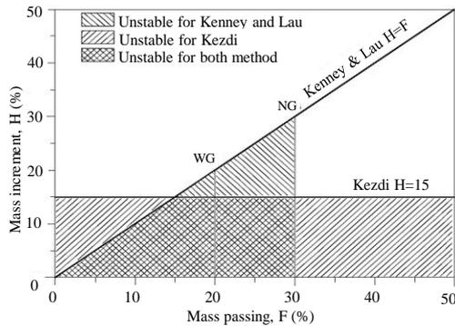
Fig.5 Synthesis of Kezdi A's and Kenney TC and Lau's criteria (Li M and Fannin RJ [11])
