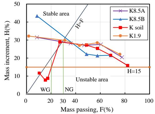
Fig.6 Internal stability assessment for Komaoka soils based on the empirical criteria [11]
