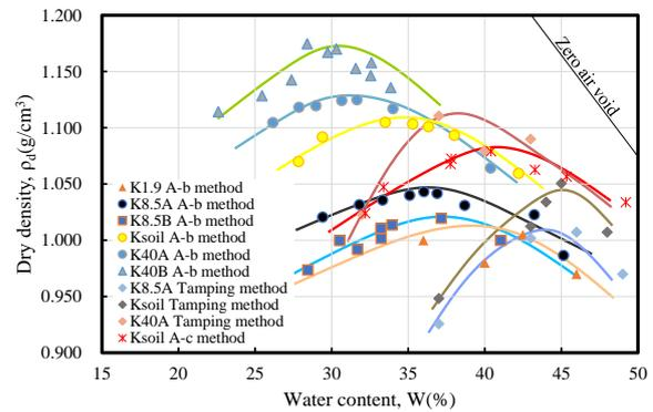
Fig.3 Compaction curves of Komaoka volcanic soils
