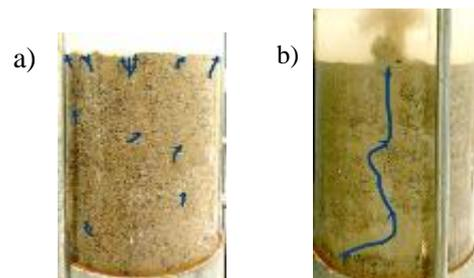
Fig.9 Observed particle migrations (a) Piping phenomenon, (b) Boiling phenomenon
