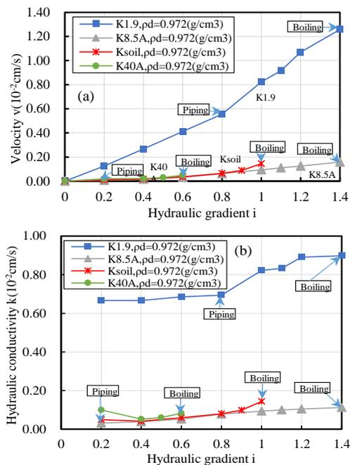
Fig.13 Test results of  $K_{soil}$ ,  $K_{8.5A}$  and  $K_{40A}$ : (a) velocity, (b) hydraulic conductivity.
