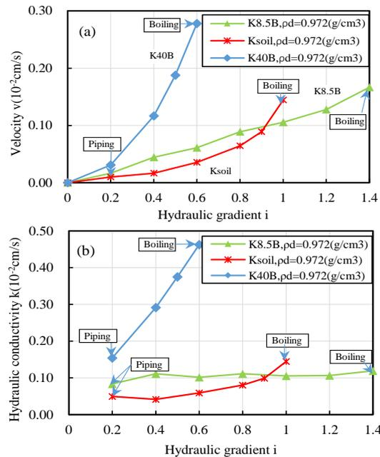
Fig.14 Test results of  $K_{soil}$ ,  $K_{8.5B}$  and  $K_{40B}$ : (a) velocity, (b) hydraulic conductivity.
