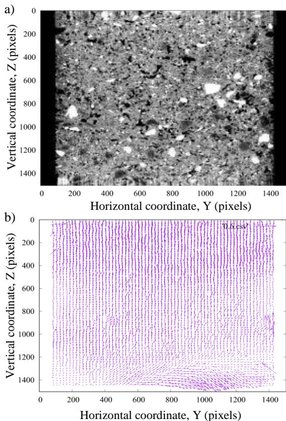
Fig.10 X-ray CT images and their DIC analysis: (a) internal image of model test, (b) particles movement at  $i=0.6$
