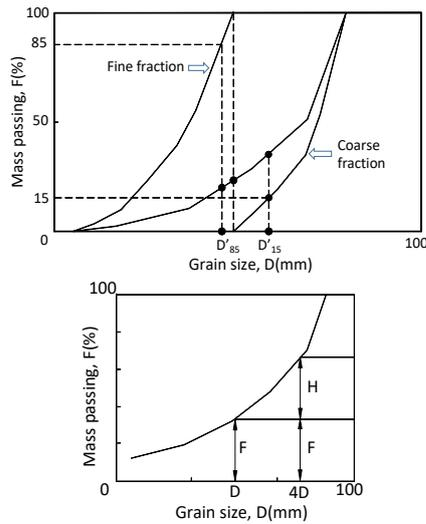
Fig.4 Stability evaluation by empirical criteria: (a) criterion by Kezdi A [7], (b) criterion by Kenney TC and Lau D [9], [10]
