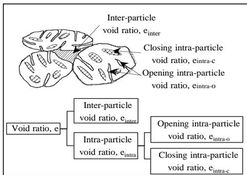
Fig. 15 Schematic of void ratio in volcanic soil (revision of [13])
