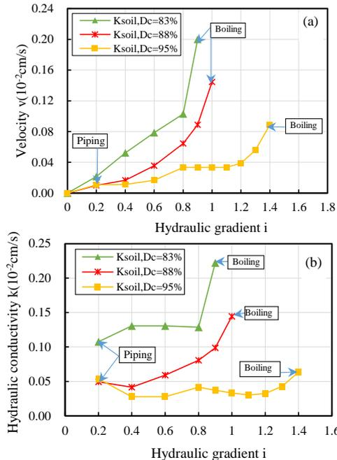
Fig.12 Change in results of  $K_{soil}$  with different compaction degrees: (a) velocity, (b) hydraulic conductivity.
