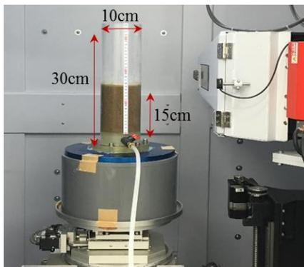
Fig.7 Test apparatus with  $\phi=100\text{mm}$  in diameter
