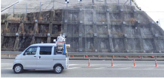
Fig.2 The MMS vehicle acquiring the point clouds of its surroundings
