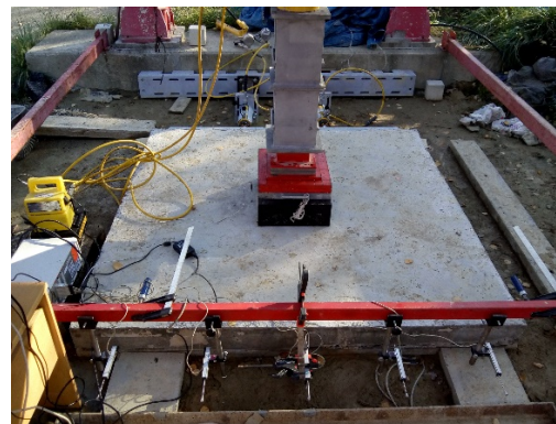
Fig.15 Positioning of the track sensors for experiment slab with horizontal and vertical load
