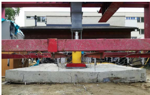
Fig.12 Deformation of the slab with vertical load
