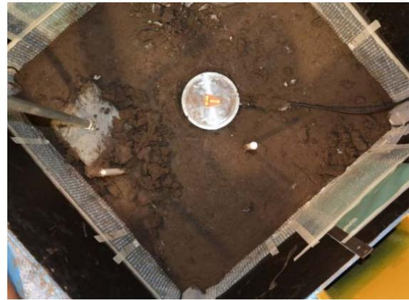
Fig.5 Installation of the soil pressure transducer
