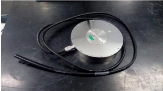
Fig.1 Soil pressure transducer
