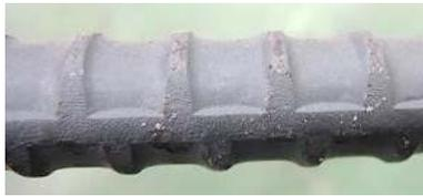
(a) Deformed bar without adhesive coating
