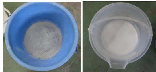
Fig.1 Compound powder (left) and liquid emulsion (right)
