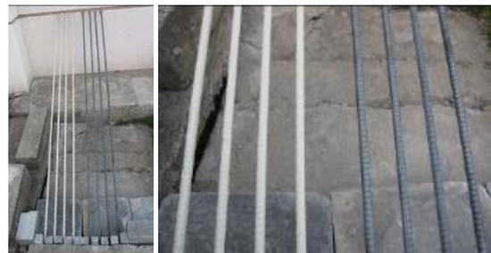
Fig.13 Field exposure of the deformed bars
