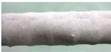
(b) Deformed bar with adhesive coating
