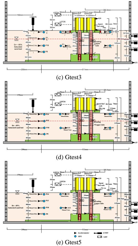
Fig. 3 Test setup and instrumentations: (a) Gtest1; (b) Gtest2; (c) Gtest3; (d) Gtest4; (e) Gtest5; the model dimensions are in centimeter and prototype dimensions (in parentheses) are in meters.
