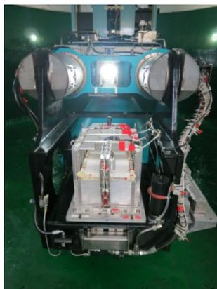
Fig. 4 Test package resting on the NCU shaker
