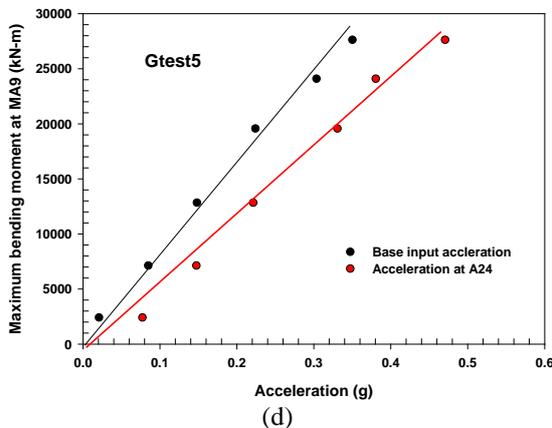
Fig. 13 Maximum bending moment measured at MA9 vs. base input acceleration and acceleration at spent fuel cask (A24): (a) Gtest1; (b) Gtest2; (c) Gtest3; (d) Gtest5
