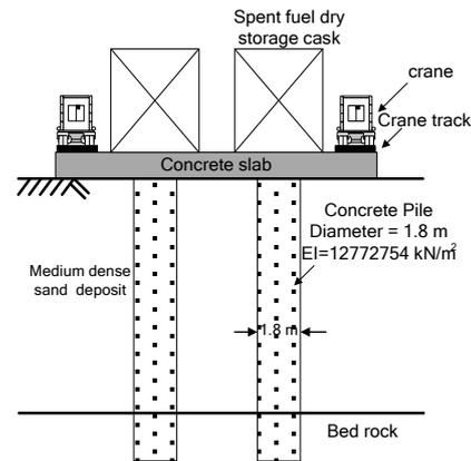
Fig. 1 Layout of spent fuel dry storage system.
