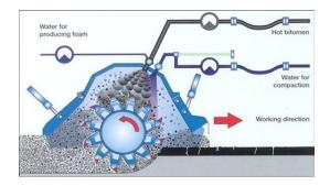
Fig.7 Foamed Bitumen mixing process [5]
