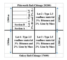
Fig.2 Site plan for segmental construction
