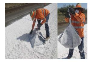
Fig.4 Matt Test carried out on site
