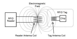
Fig.1 Basic RFID system
