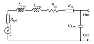
Fig. 4 Equivalent circuit of an inductive loop antenna
