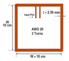
Fig. 5 Physical dimension of the loop antenna
