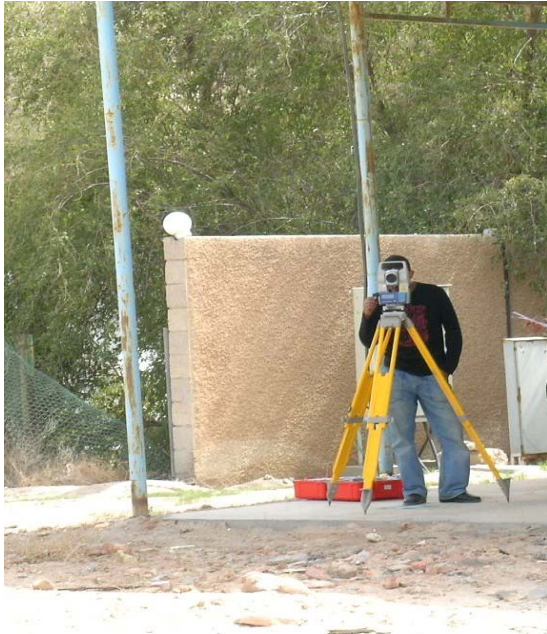
Fig. 4. Recording readings by total station survey.
