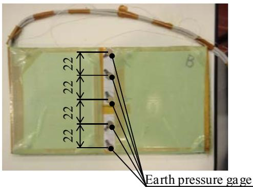
Photo. 2 Earth pressure gage (left hand side) and displacement gage (right hand side)
