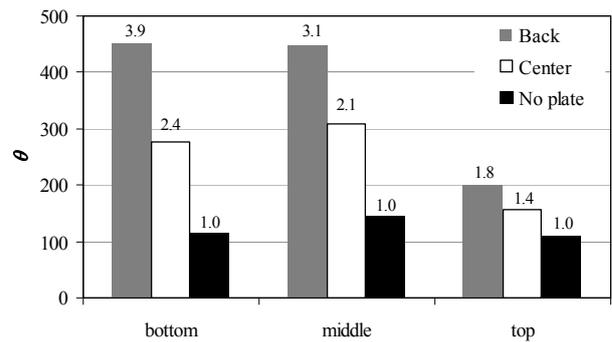
Fig. 8 Relative effect of resistance linked with plate position,  $\theta$  defined as a gradient in the relationship between  $P_H$  values normalized by  $\gamma H^2 B/2$  and the relative horizontal displacement  $\delta h$  normalized by the depth of the block  $D$
