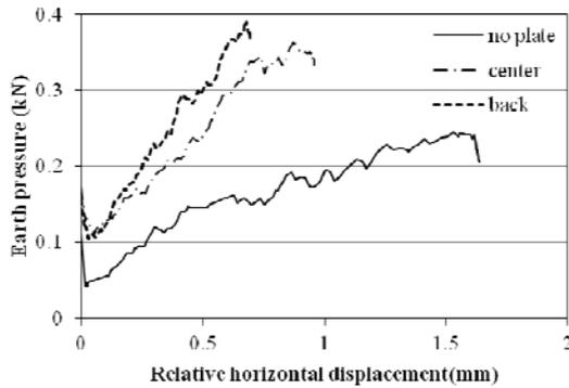
Fig. 7 Relationship between total rear earth pressure and relative horizontal displacement at the bottom block
