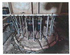
Fig.13 Loader with hydraulic jack
