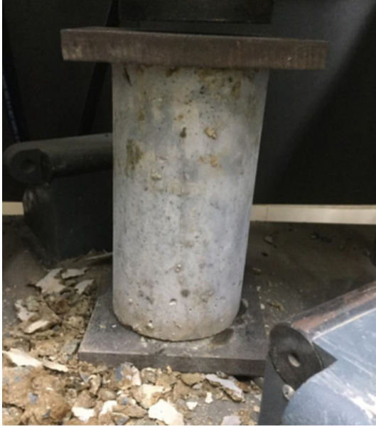
Fig. 6 Sample Concrete mixed with Bauxite Laterite Soil Substitution
