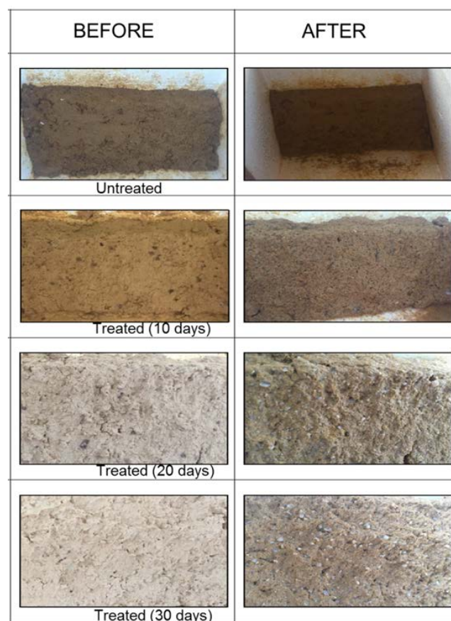
Fig. 6 Slope surface before and after rain simulation
