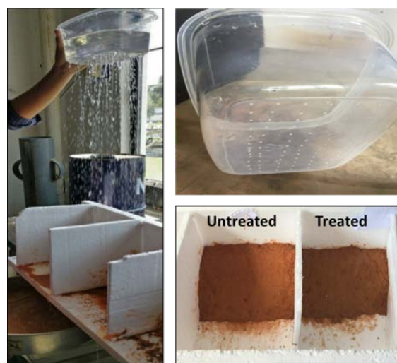
Fig. 4 Rainfall simulation using soil slope models of untreated and treated samples
