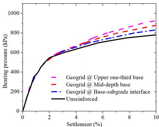
Fig. 6. Bearing pressure vs. settlement ratio of unreinforced and reinforced unpaved roads
