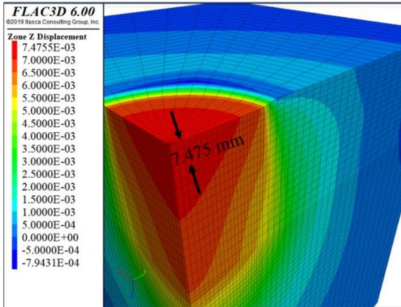
Fig. 2. Vertical displacement contours of the unreinforced unpaved section
