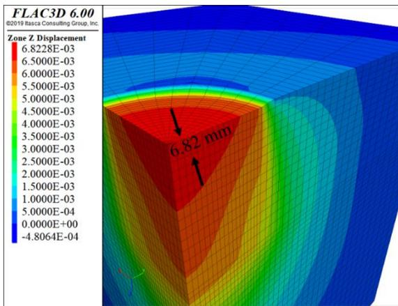
Fig. 3. Vertical displacement contours of the reinforced unpaved section
