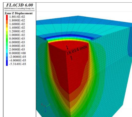
Fig. 5a Unreinforced section (subjected to loading of 700 kPa)
