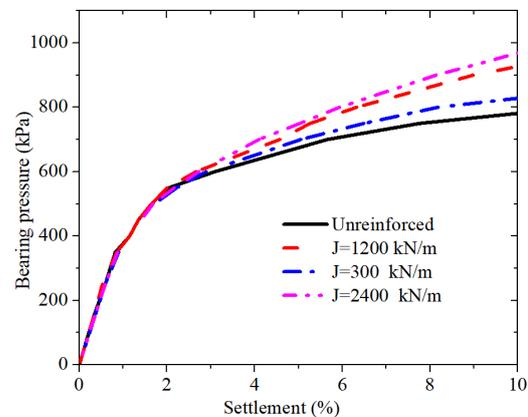
Fig. 7. Bearing pressure vs. settlement ratio of pavements reinforced with various geogrid axial stiffness
