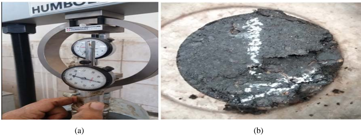
Fig.4 (a) Breaking the asphalt molds on the Marshal machine. (b) The form of asphalt molds after breaking.
