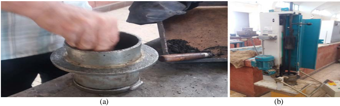
Fig.3 (a) Compacted the mixture into the mold. (b) Compaction of the asphalt molds mechanically.
