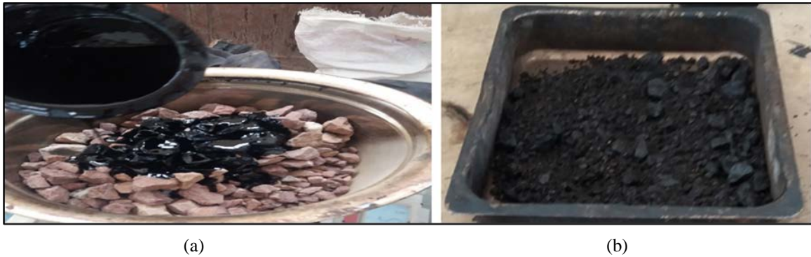
Fig.2 (a) Adding the binder of asphalt to mix aggregates; (b) The mixture of asphalt after mixing.
