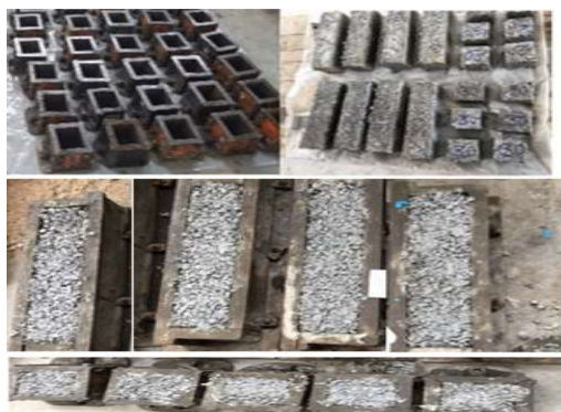
Fig.2 Casting of some specimens
