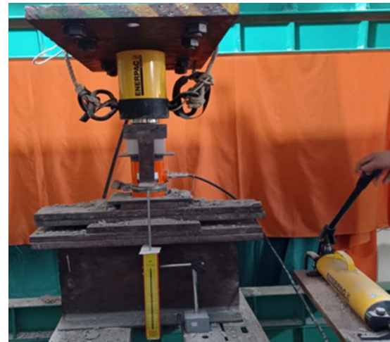
Fig 3. Unconfined Compression Strength test
