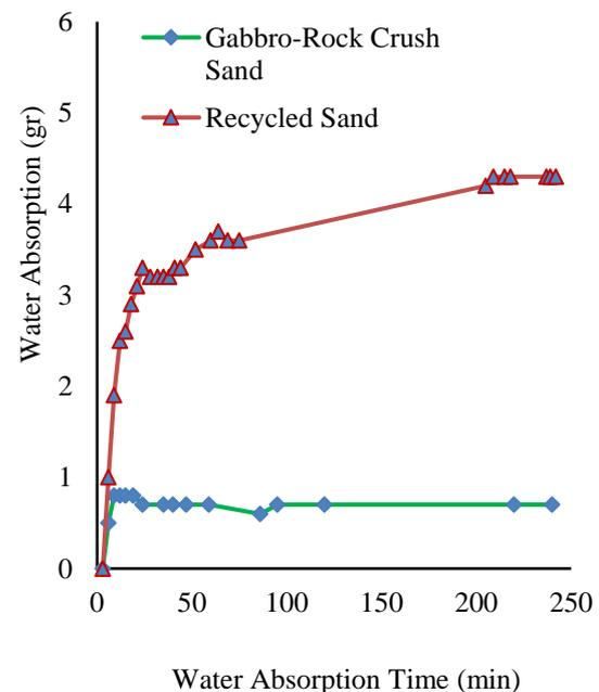
Fig.6 Water absorption of fine aggregates immersed in water.
