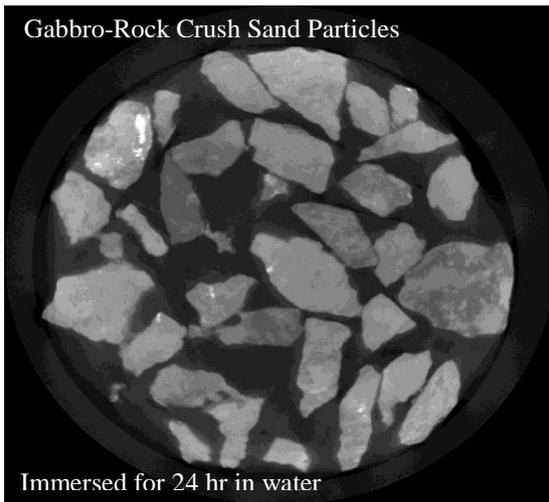
Fig.7 X-ray CT scanned image of gabbro-rock crush sand immersed in water for 24 hours
