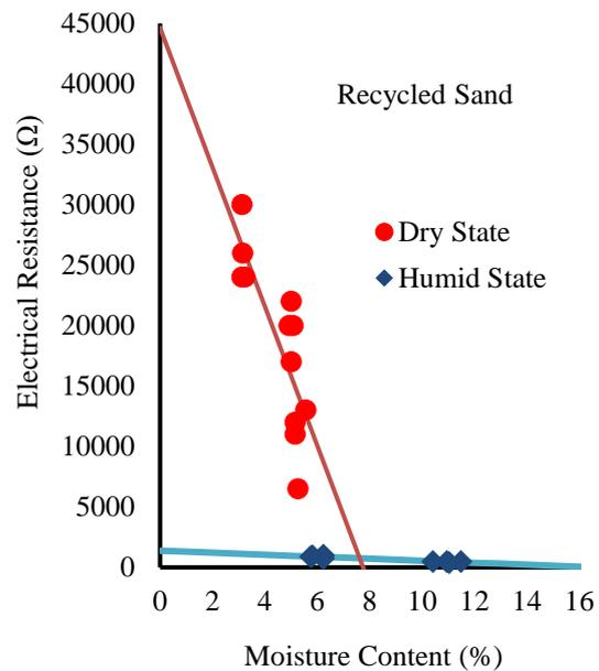
Fig.4 Electrical conductivity test result for recycled sand
