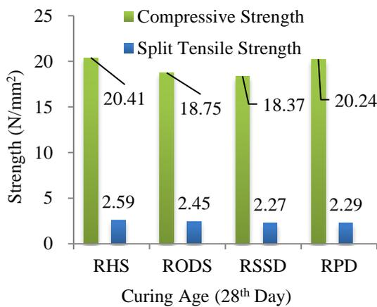
Fig.13 Compressive and split tensile strength of recycled sand mortar specimens
