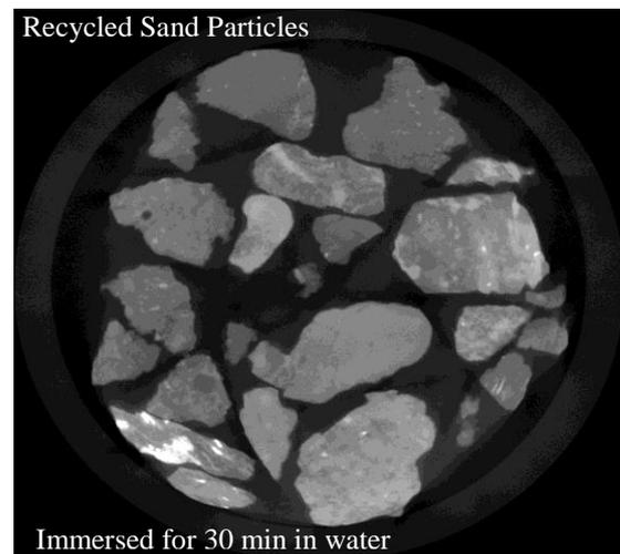
Fig.11 X-ray CT scanned image of recycled sand immersed in water for 30 minutes
