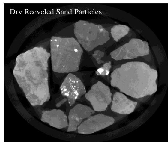
Fig.12 X-ray CT scanned image for the dry state of recycled sand
