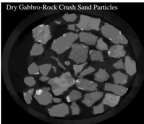
Fig.9 X-ray CT scanned image for the dry state of gabbro-rock crush sand.
