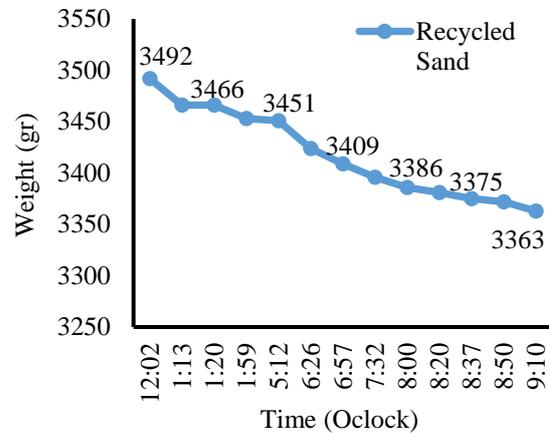
Fig.2 Weight loss of recycled sand in an incubator under 55 °C constant.
