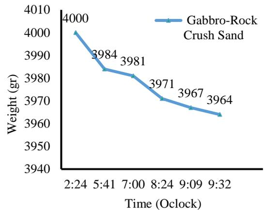
Fig.3 Weight loss of gabbro-rock crush sand in ball mill method
