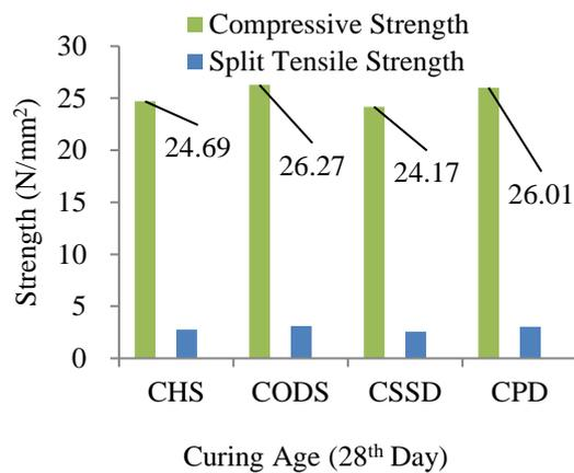
Fig.14 Compressive and split tensile strength of gabbro-rock crush sand mortar specimens
