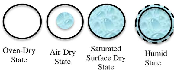
Fig.1 Different moisture states of FA particles
