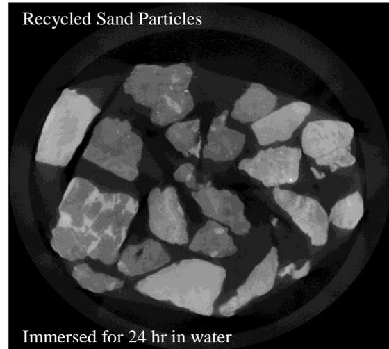
Fig.10 X-ray CT scanned image of recycled sand immersed in water for 24 hours
