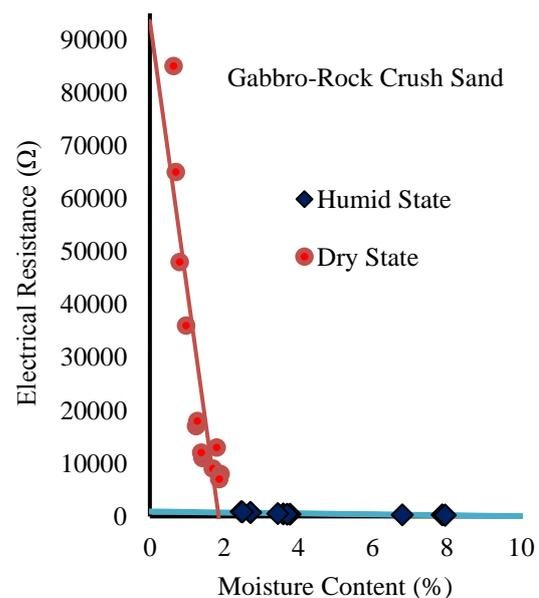
Fig.5 Electrical conductivity test result for gabbro-rock crush sand.
