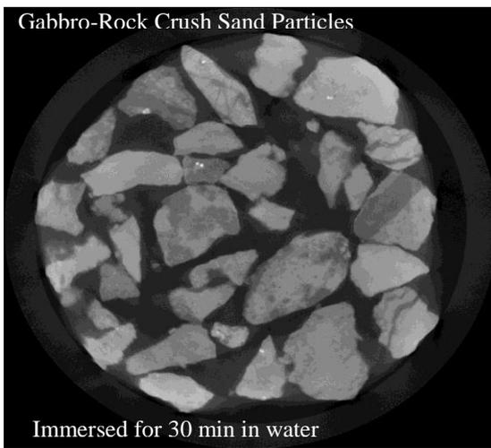
Fig.8 X-ray CT scanned image of gabbro-rock crush sand immersed in water for 30 minutes
