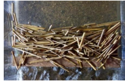
Fig.7 Top view of piece accumulation at the pipe culvert bridge
