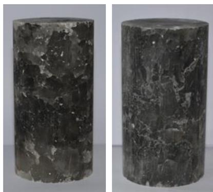
Fig.1: Manufactured salt samples
