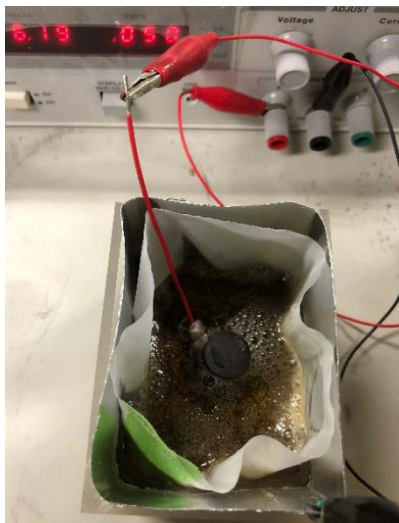
Photo. 1 A simulated flexible container bag (test equipment)
