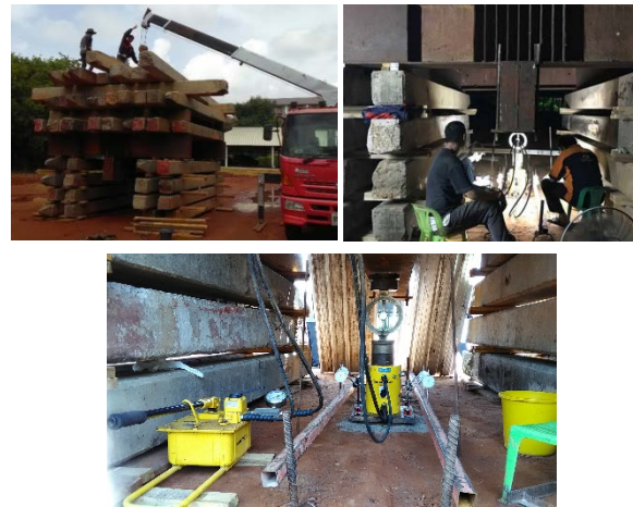
Fig.13 Plate load test installation
