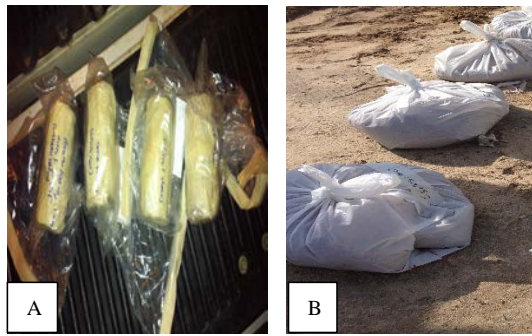
Fig. 4. Indicating to undisturbed (A) and disturbed (B) soil samples.
