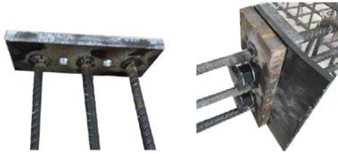
Fig. 3 Connection on the bottom reinforcement steel of the beam [5]
