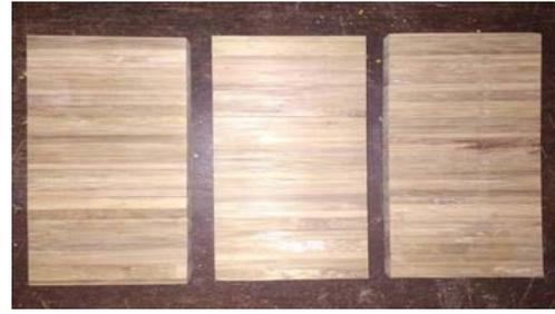
Fig.3 Specimens creep shear test of glued-laminated bamboo
