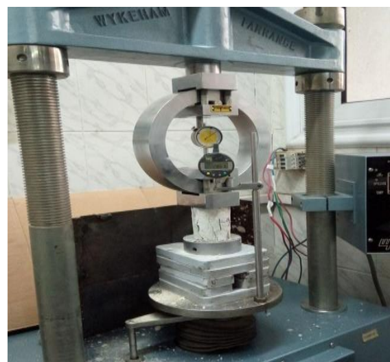
Fig.2 Sample ready for testing for unconfined compressive strength
