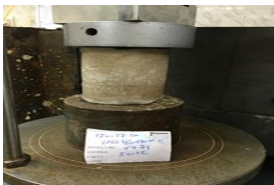
Fig. 3 shows the set up for measurement of vertical and lateral deformations
