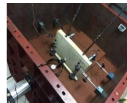
(c) Proving Ring, LDVTs and Pneumatics
