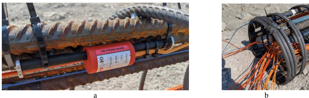
Fig. 3 Vibrating wire strain gauge linked to a rebar (a) and cables exiting the top of the steel cages (b)
