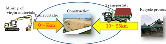
Fig. 7 Overview of recycling construction sludge as ground material
