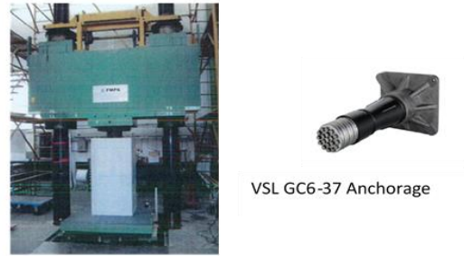
Fig.7 Experimental test setup for VSL GC6-37 anchorage type [11]
