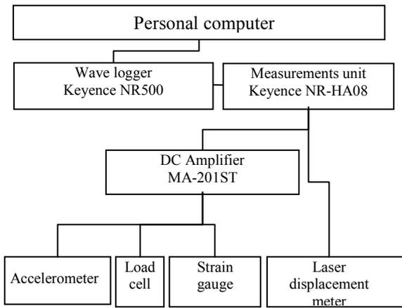
Fig. 7 Measurement system
