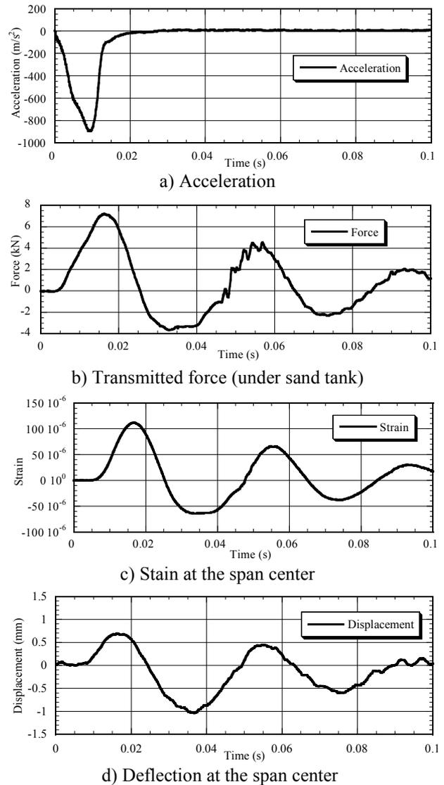
Fig. 8 Time histories of measured data (Sand, span length 1.8m, falling height 2.0m)
