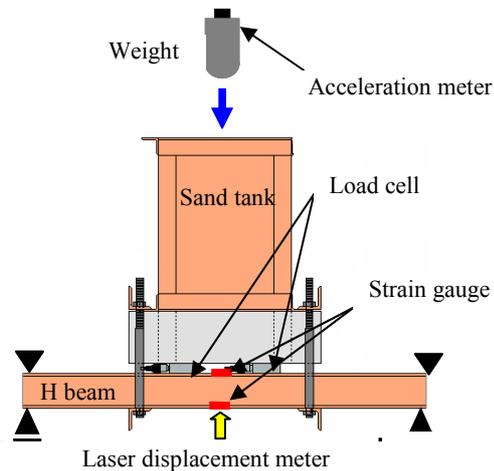
Fig. 6 Measurement devices and their locations
