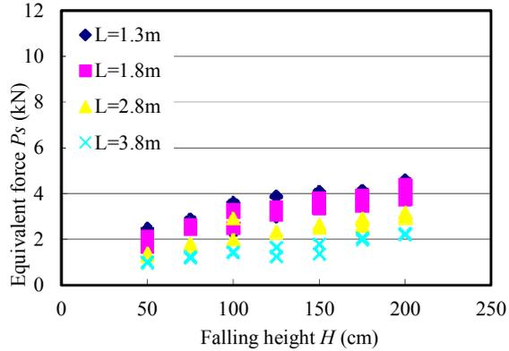
c) Falling height and equivalent force  $P_s$
