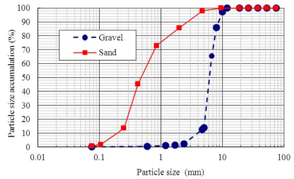
Fig. 5 Particle size accumulation curve
