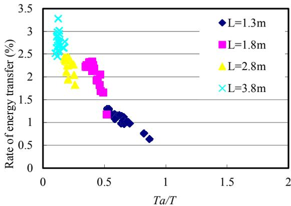
Fig. 14 Relationship between  $T_a/T$  and rate of energy transfer to beam from falling weight (sand)
