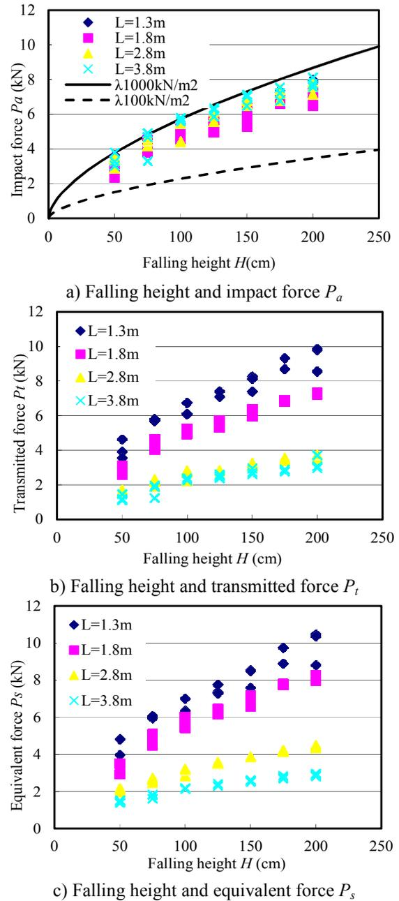
Fig. 11 Relationship between falling height and various maximum forces for sand
