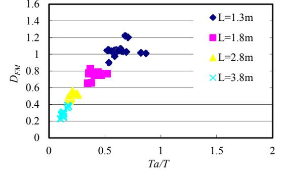
(b) Relationship between  $T_a/T$  and dynamic multiplication factor  $D_{FM}$  ( $T_a$ : duration of impact force,  $T$ : the first natural period of beam)
